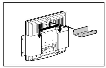
Figure 2-20. Placing the power supply tray
